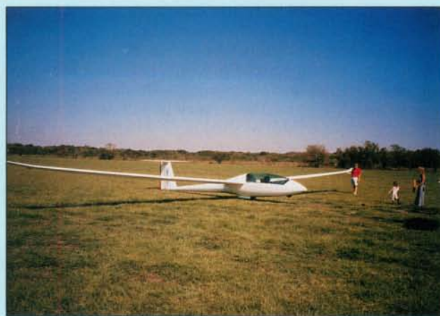
The one piece canopy and lowered nose provide the pilots with excellent visibility. Note the fixed nose wheel, and the large retractable main wheel and doors under the wing. The tail wheel exists, but is buried in the runway grass.
