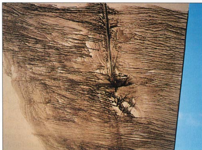
Another view of the wing bottom surface oil flow patterns after the 55 kt test flight.
