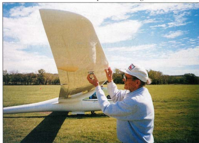
The author performing chordwise waviness measurements with a 2 inch long wave gage on N117GV's wing lower surface near its swept back wing tip.
