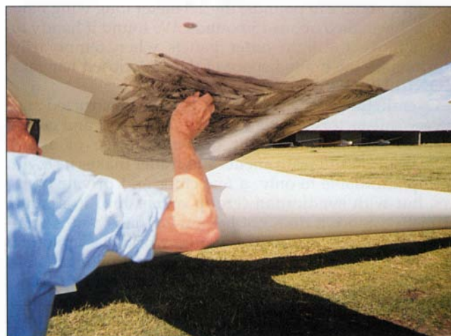
The author using an ordinary paint brush to apply darkened 10W-40 motor oil to the aft 60% of a 42 inch wide section of the wing bottom surface, before the oil flow test flight.
