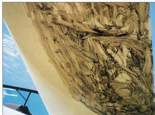
The as-brushed bottom surface oiled section of the wing before takeoff. Note that the factory installed spanwise turbulator at .73 chord extends about eight inches into both the inboard and outboard portions of the oiled area. Also that a 26 inch long section of the turbulator in the central part of the oiled area was removed to see if any separation bubble did indeed exist in flight.
