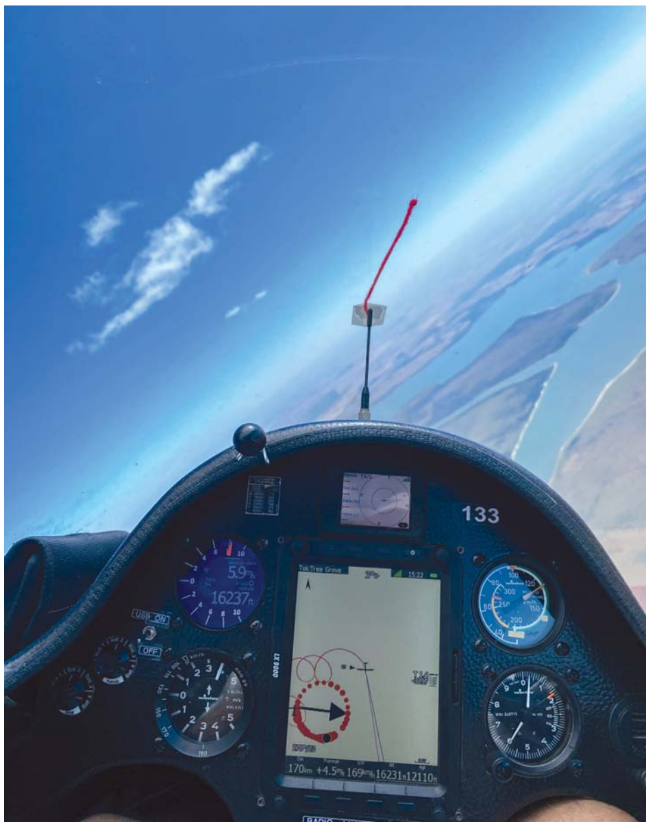
Steep banks at slow airspeed mean smaller circles (i.e. smaller radii). Photo by Roy Bourgeois.
